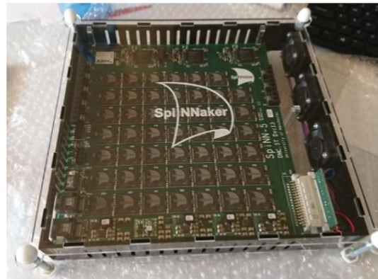
SpiNN 5: 48 SpiNNaker chips
