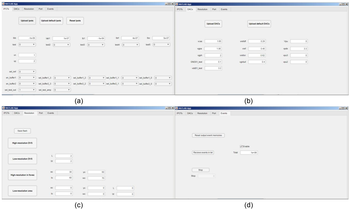
Figure 9. Matlab GUI for the sensor configuration. (a) Tab for Ipots configuration, (b) tab for voltage biases configuration, (c) tab for sensor resolution configuration, and (d) tab for capturing output events using the STM32 microcontroller.
